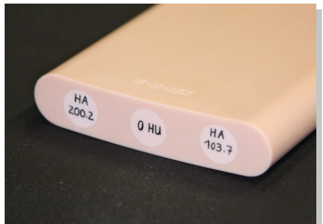
QRM-Bone in the Bone Calibration Phantom
