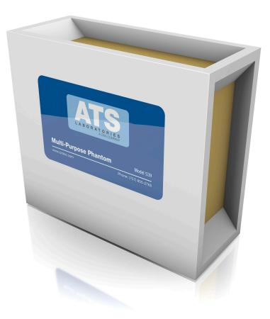
The Model 539 Multipurpose phantom is an easy, comprehensive means of evaluating imaging systems over the full range of clinical imaging frequencies (2 MHz to 18 MHz).
