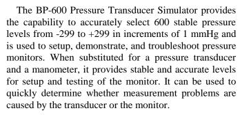
The stability of the BP-600 is significantly better than techniques that produce an electrical output by using a transducer to measure the pressure of a fixed volume of air. Under these conditions, the pressure applied to the transducer is also affected by temperature as defined by the Ideal Gas Law. The BP-600 is designed to minimize thermal instability and thus provides an output that is more stable than pressure transducer systems in common use.
