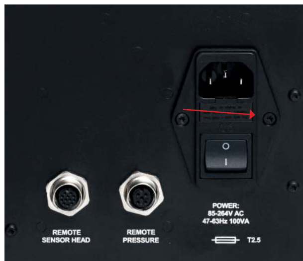
Figure 25 Power Supply Fuse Replacement
