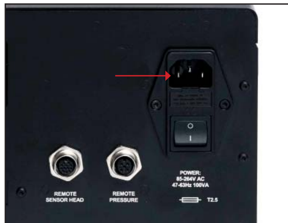
Figure 3 Power Supply Input
