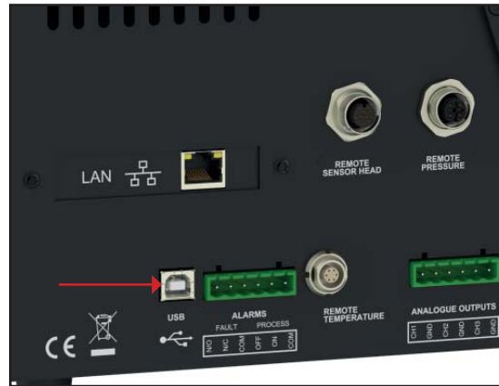
Figure 8 USB Port Connection
