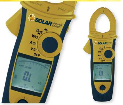
The new Solar Power Clamp is a clamp meter capable of measuring AC and DC circuit power, in addition to true RMS voltage and current, resistance & continuity, diode check, capacitance, harmonic distortion and power factor.
