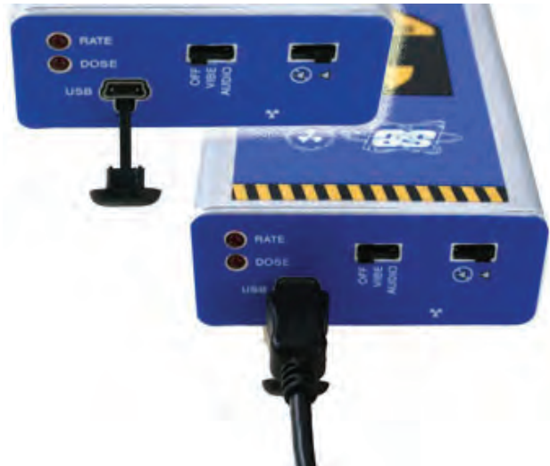
Fig 5. The Sentry EC - Unplug the mini-USB cap from the USB port and connect the mini-USB cable
