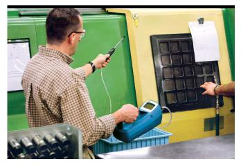
P-Trak Ultrafine Particle Counter and accessories includes: Telescoping Sample Probe, Shoulder Strap, Inlet Screen, Spare Wicks (2), Alkaline Batteries, Alcohol Fill Capsule with Storage, Jack Steer, Spare Wicks (c), Atkane batteries, Alcolor Filters (2), Carrying Case, TrakPro™ Software, Computer Cable, Operation and Service Manual, Calibration Certificate, and Two-year Warranty.
