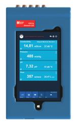
The HDC75 display and control unit was developed with the busy biomed technician in mind. The combination of a touch screen and the Windows 10 operating system opens up new possibilities in daily tasks i.e repairing and calibrating medical instruments. Printing, sending reports via eMail, even online databases are all now made possible.
